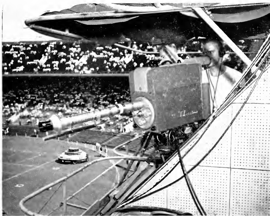
When WFIL-TV's camera is equipped with the Zoomar lens, this lens is used for approximately 75 per cent of the game coverage. It is particularly effective on long passes and long runs.
